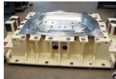
The coated deep-drawing tools result in a significant increase in productivity.
